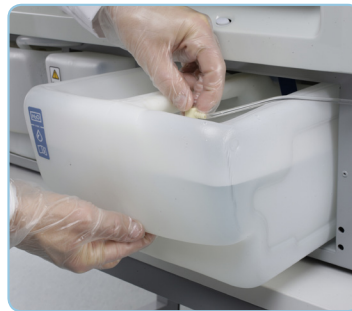
The analyzer is self-contained with no need for external water or drainage connections, which makes the analyzer quick and easy to install.
