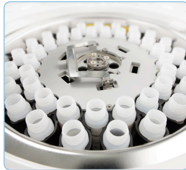
Reagent disk for 42 reagents. The reagent usage and expiry date are automatically monitored in real-time.
